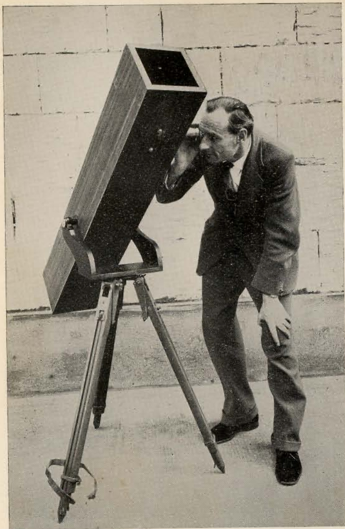
A simply constructed 6 inch Newtonian telescope details of which are given in Chapter XV. The telescope can be mounted on an ex-Government tripod like this one or for greater stability, a four-legged stand can be easily made.
